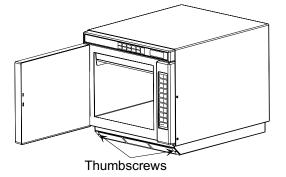
Removing Air Intake Filter
